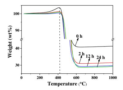
**Fig. 7** TGA curves of sample A1800-4-5 after different time acid-washing, carried out in air with a heating rate of 10 °C/min.
