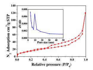
Fig. 1 Nitrogen sorption isotherm and pore size distribution of core/shell Fe@CNCs.
