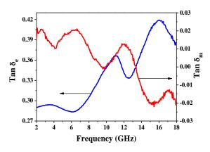
Fig. 11 Dielectric tangent loss (tan  $\delta_e$ ) and magnetic tangent loss (tan  $\delta_m$ ) of core/shell Fe@CNCs in 2-18 GHz.
