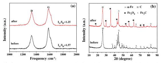
Fig. 8 Raman spectra (a) and XRD patterns (b) of core/shell Fe@CNCs before and after thermal annealing in air.
