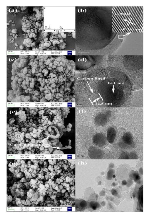
Fig. 5 SEM (a, c, e and g) and TEM (b, d, f and h) images of core/shell Fe@CNCs, A1800-4-5 (a, b), A1800-2-15 (c, d), A2400-4-15 (e, f) and A1800-4-15 (g, h), inset in SEM image (a) is the corresponding EDS spectrum.
