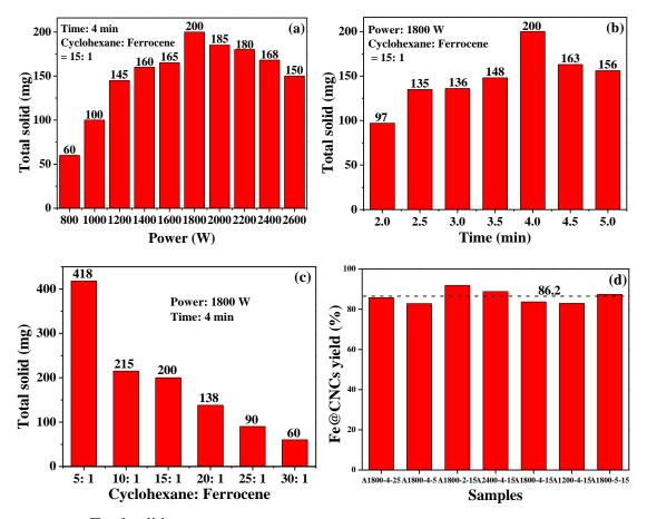
**Fig. 2** Total solid (a, b and c) of the raw product in each batch under different working conditions and Fe@CNCs yield (d).
