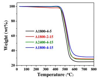
**Fig. 6** TGA curves of different core/shell Fe@CNCs in air with a heating rate of 10 °C/min, the Fe content of the sample A1800-4-5, A1800-2-15, A2400-4-15 and A1800-4-15 are calculated to be 17.5, 20.1, 19.6 and 22.0 wt%, respectively.
