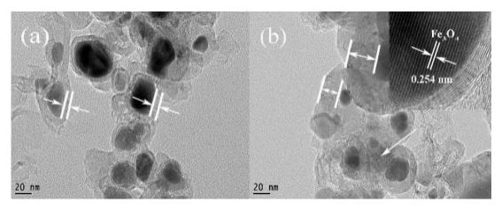
Fig. 9 High resolution TEM images of core/shell Fe@CNCs before (a) and after (b) thermal annealing in air.
