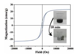
Fig. 10 Magnetic hysteresis loop of core/shell Fe@CNCs, take sample A1800-4-5 as an example.
