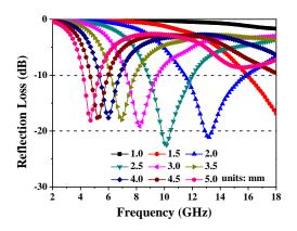
Fig. 12 Reflection loss of core-shell Fe@CNCs with absorber thickness of 1-5 mm.
