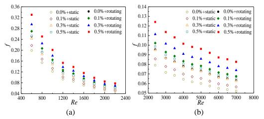
Figure 18 Resistance coefficients of nanofluids at different Reynolds numbers, (a) laminar flow; (b) turbulent flow
