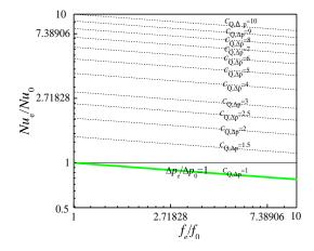
Figure 10 Performance evaluation plot for exergy efficiency under the same pressure drop
