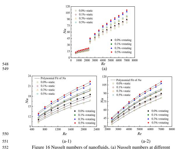
Figure 16 Nusselt numbers of nanofluids, (a) Nusselt numbers at different Reynolds numbers; (a-1) fitted curves at laminar flow; (a-2) fitted curves at turbulent flow
