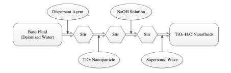
Figure 1 Preparation procedure of TiO<sub>2</sub>-H<sub>2</sub>O nanofluids by a two-step method
