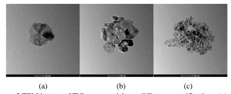
Figure 2 TEM images of  $TiO_2$  nanoparticles at different magnifications, (a)  $\longmapsto$  20nm; (b)  $\longmapsto$  50nm; (c)  $\longmapsto$  100nm
