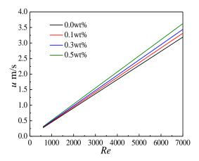
Figure 15 Changes of velocity with nanoparticle mass fraction under different Reynolds numbers
