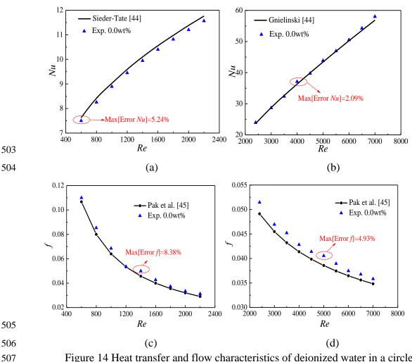
Figure 14 Heat transfer and flow characteristics of deionized water in a circle tube, (a) *Nu*-laminar flow; (b) *Nu*-turbulent flow (c) *f*-laminar flow; (d) *f*-turbulent flow
