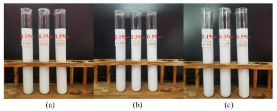
Figure 3 Nanofluids at different times, (a) before laying up; (b) laying up for 3 days; (c) laying up for 7 days
