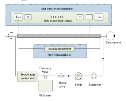
Figure 5 Schematic diagram of the experimental system
