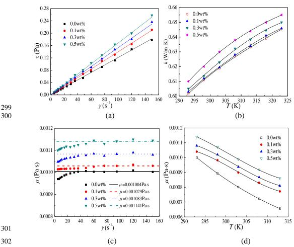
Figure 4 Thermophysical properties of  $TiO_2$ -water nanofluids (a) Newtonian-fluids characteristics at  $T_f$  = 293 K; (b) thermal conductivities; (c) viscosity changes with shear rates at  $T_f$  = 293 K; (d) viscosity changes with temperatures [33]
