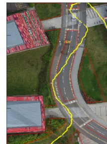
Fig. 7. Multipath affecting the GNSS receiver. Actual walk went along the left walkway.
