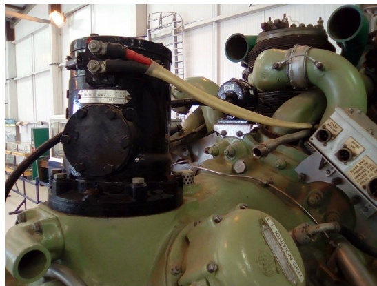
Fig. 3. 1kW at 28Vdc engine-driven DC generator, stored in the Shuttleworth Museum (Biggleswade, UK).
