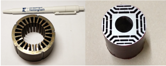
Fig. 9: Stator and rotor lamination stacks before winding and assembling (pictures are not shown in the same scale)
