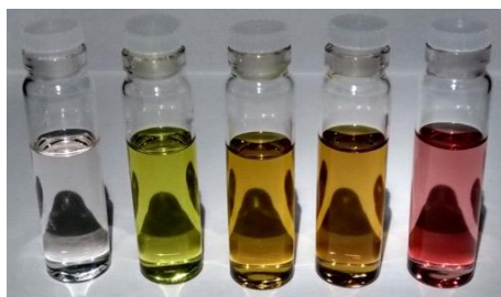
Figure 3. Solutions of thionated NDIs in dichloromethane solutions. Left to right: NDIS 0 , NDIS 1 , cis - NDIS 2 , trans - NDIS 2 , NDIS 3 .
