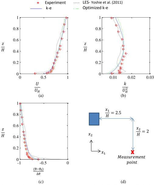
Figure 14 Vertical profiles of flow parameters along a vertical line far from the building in high speed region at  $\frac{x_1}{H} = 2.5$  and  $\frac{x_2}{H} = 2$ : (a) streamwise velocity  $\frac{U}{U_H}$ , (b) turbulent kinetic energy  $\frac{k}{U_H^2}$ , (c) non-dimensional temperature  $\frac{(\theta - \theta_f)}{\Delta \theta}$ , (d) measurement position
