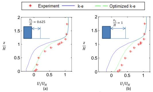
Figure 11 Vertical distribution of the streamwise velocity  $\frac{U}{U_H}$  in the wake region behind the building at: (a)  $\frac{X_1}{H} = \mathbf{0}.625$ , (b)  $\frac{X_1}{H} = \mathbf{1}$
