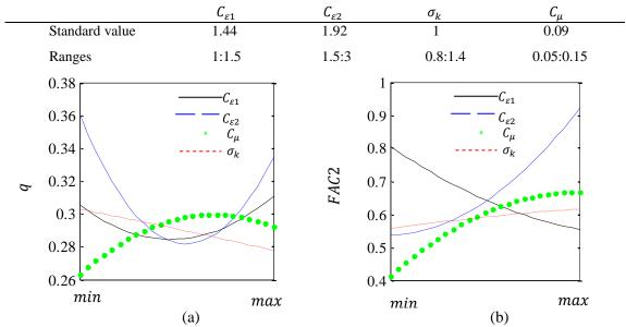
Figure 6 Variation of the validation metrics for the streamwise velocity component for isolated building case study: (a) hit rate q, (b) FAC2
