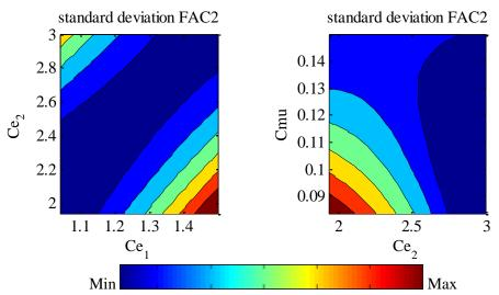
Figure 10 Plot of the standard deviation of the FAC2 for streamwise velocity in the optimization process
