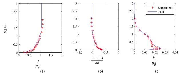
Figure 5 Inflow boundary condition for (Yoshie et al, 2011): (a) velocity, (b) temperature, (c) turbulent kinetic energy
