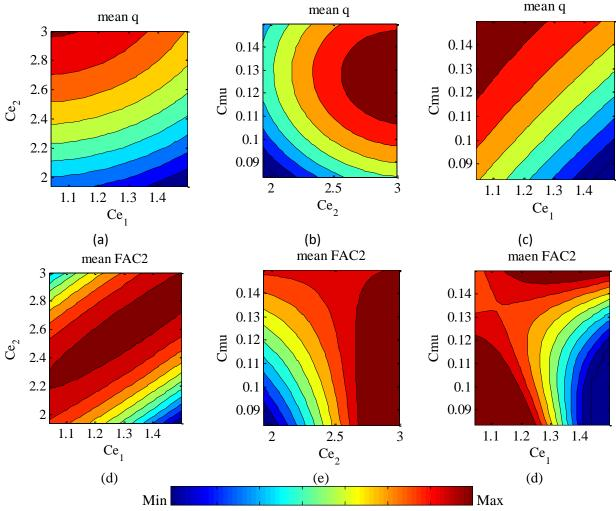
Figure 9 Variation of the mean value of the validation metrics for the streamwise velocity component and the closure coefficients during the optimization process
