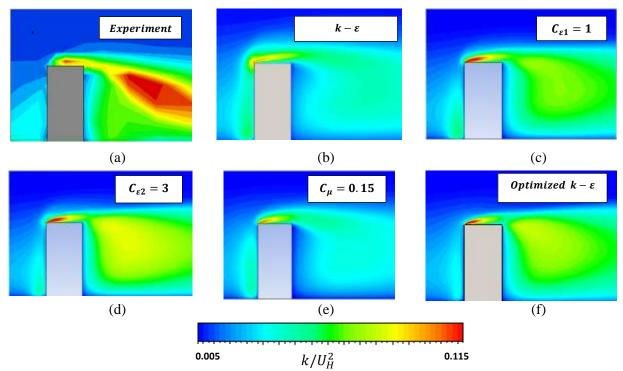
Figure 7 Contours of the turbulent kinetic energy: (a) experiments by Yoshie et al (2011), (b)  $k - \varepsilon$ , (c)  $C_{\varepsilon 1} = 1$ , (d)  $C_{\varepsilon 2} = 3$ , (e)  $C_{\mu} = 0.15$ , (f) optimized coefficients
