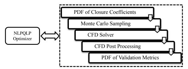
Figure 2 Schematic of the stochastic optimization of the closure coefficients
