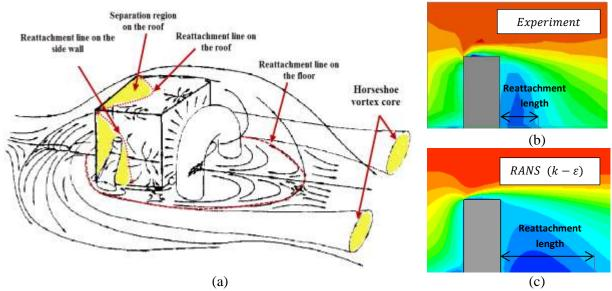
Figure 1 (a) Flow visualization around an isolated building (Hunt et al, 1978). Streamwise velocity distribution around an isolated building for (b) experiment by Yoshie et al (2011), (c) RANS turbulence mode
