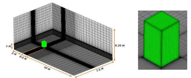
Figure 4 Computational domain and grid arrangement
