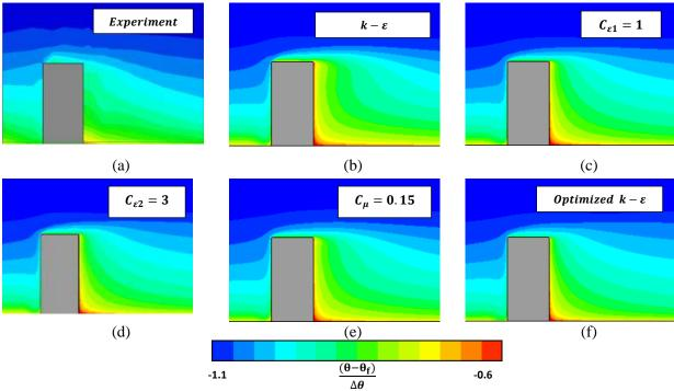
Figure 8 Distribution of the non-dimensional temperature  $\frac{(\theta - \theta_f)}{\Delta \theta}$ : (a) experiments by Yoshie et al (2011), (b)  $k - \varepsilon$ , (c)  $C_{\varepsilon 1} = 1$ , (d)  $C_{\varepsilon 2} = 3$ , (e)  $C_{\mu} = 0.15$ , (f) optimized coefficients
