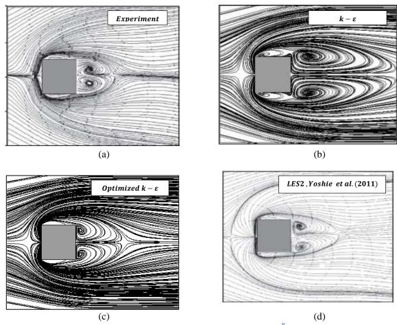
Figure 12 Horizontal distribution of the streamlines near the ground ( $\frac{X_3}{H} = 0.025$ ): (a) experiment by Yoshie et al (2011), (b) default  $k - \varepsilon$  closure coefficients, (c) modified  $k - \varepsilon$  closure coefficients, (d) LES-2 from (Yoshie et al, 2011)
