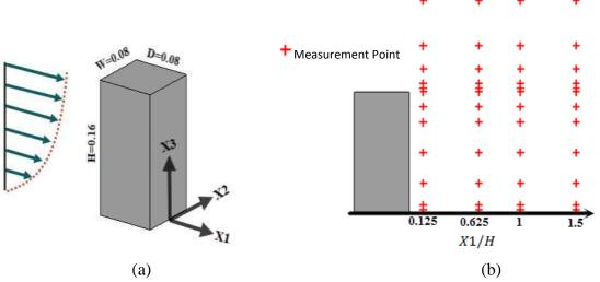
Figure 3 Schematic of Yoshie et al (2011) experiment: (a) bluff body dimensions, (b) measurement points
