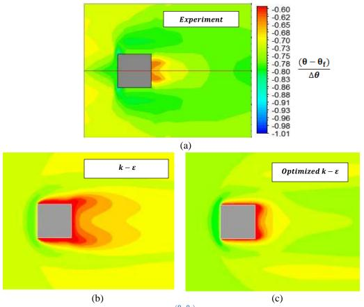
Figure 13 Contours of the temperature distribution  $\frac{(\theta - \theta_f)}{\Delta \theta}$  near the ground surface: (a) experiment by Yoshie et al (2011), (b) default  $k - \varepsilon$  closure coefficients, (c) modified  $k - \varepsilon$  closure coefficients
