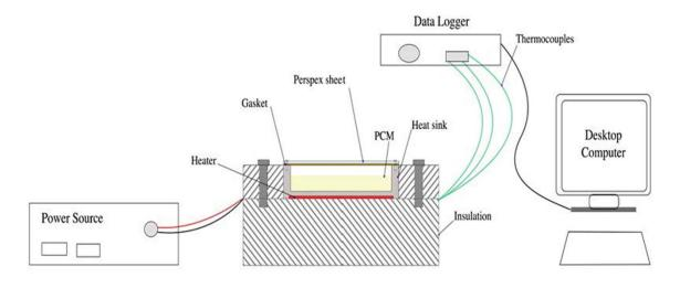
Figure 1a-Shematic diagram of experimental setup.
