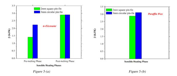
Figure 5-Comparison of thermal capacity of heat sinks (a) n-eicosane (b) paraffin wax
