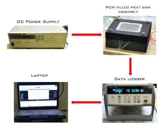
Figure 1b-Line flow of experimental facility.
