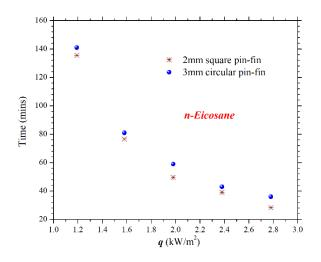
Figure 3-comparison of latent heating phase completion time.
