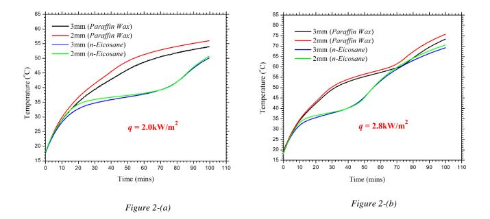
Figure 2-Comparison of heat sinks base temperature for paraffin wax and n-eicosane. (a)  $q = 2.0 kW/m^2$  (b)  $q = 2.8 kW/m^2$
