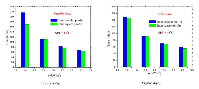
Figure 4-Comparison of enhancement in operation time. (a)  $SPT = 65^{\circ}C$  (b)  $SPT = 45^{\circ}C$ .
