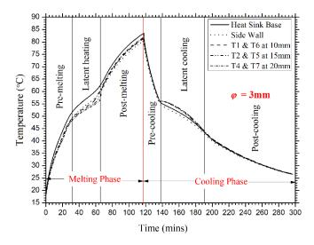
Figure 8-Charging and discharging cycle of  $\varphi = 3mm$  pin-fin heat sink at 2.8kW/m<sup>2</sup>.
