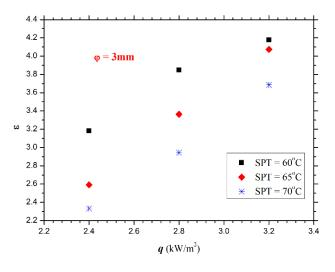
Figure 13- Comparison of enhancement ratios between different SPTs for 3mm pin diameter pin-fin heat sink.
