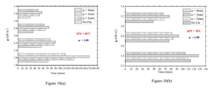
Figure 10- Comparison of enhancement time between various configurations of round pin-fin heat sinks (a)  $SPT=60^{\circ}C$  (b)  $SPT = 70^{\circ}C$
