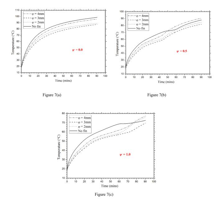
Figure 7- Comparison of fin diameter of different volumetric fractions of PCM at  $2.8kW/m^2$  (a)  $\psi = 0.0$  (b)  $\psi = 0.5$  (c)  $\psi = 1.0$
