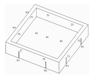
Figure 4-Positoins of thermocouples.
