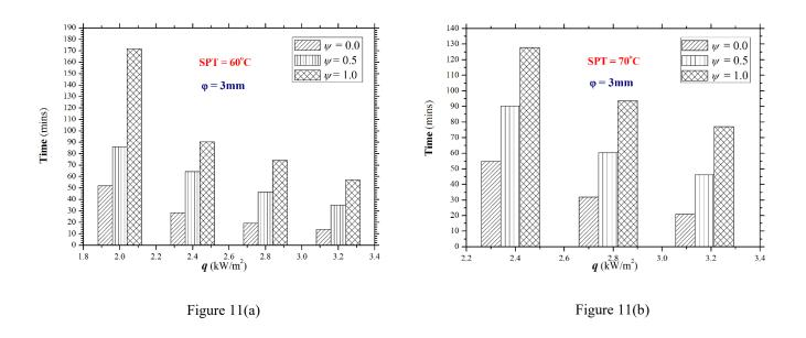
Figure 11- Comparison of enhancement time for different volumetric fraction of PCM of  $\varphi = 3mm$  pin-fin heat sink (a) SPT=60°C (b)SPT = 70°C
