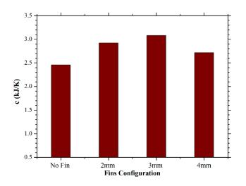
Figure 14-Comparsion of heat capacity for different configurations of round pin-fin heat sinks.
