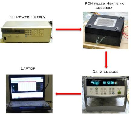
Figure 1-Flow diagram for present experimental HSU.
