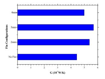
Figure 15-Comparsion of thermal conductance for different configurations of round pin-fin heat sinks.
