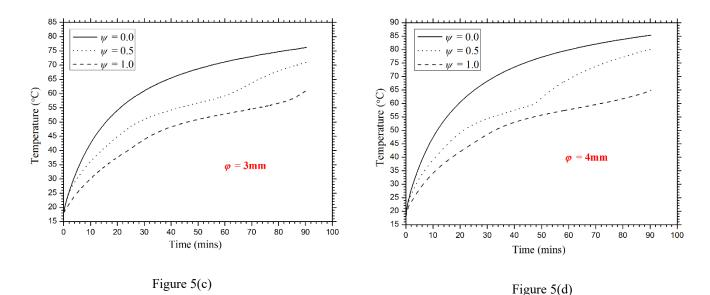
Figure 5- Comparison of heat sinks base temperature at different volumetric fractions of PCM (a) No fin (b)  $\varphi = 2mm$  (c)  $\varphi = 3mm$  (d) $\varphi = 4mm$
