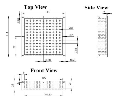
Figure 2- Two dimensional projections of 3mm pin diameter heat sink.
