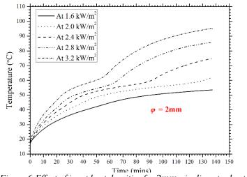
Figure 6-Effect of input heat densities for 2mm pin diameter heat sink.
