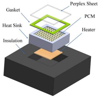
Figure 3-Assembly drawing of PCM based heat sink.
