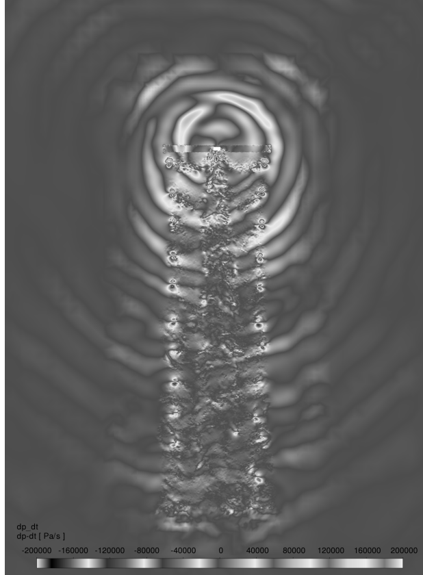
Fig. 10 Snapshot of pressure dilatation dp/dt on the axial plane.
