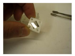
Fig. 9.. A 10  $\times$  10  $\,\mathrm{mm^2}$  zinc-blende free-standing GaN substrate prepared for further epitaxy.
