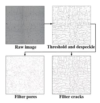
Figure 6 - Identification of the increased cracking and porosity regions in the 'island' intersections. Note that the cracking has a distinct directionality at  $0^{\circ}$  and  $90^{\circ}$  to the 'island' borders, aligned with the laser scan vectors
