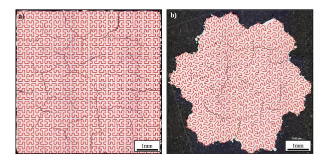
**Figure 9** - Backscatter electron micrographs in the *XY* plane of the Hilbert 100W 600mm.s<sup>-1</sup> sample showing: (a) bidirectional crack origin at intersection between fine and coarse equiaxed grains; (b) high angle cracking with (inset c) some sub-micron size precipitates identified along the crack surface
