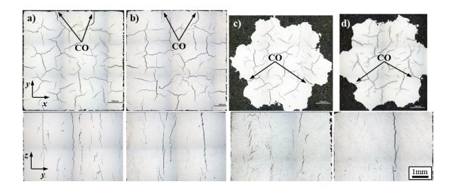
**Figure 8** - (a) Hilbert [100W, 600mm.s<sup>-1</sup>] and (b) Peano-Gosper [75W, 600mm.s<sup>-1</sup>] scanning strategies approximately overlaid on to the deposits formed via SLM. Note that the cracking does not seem to follow the scan vectors as with the long vector length samples. Further, cracks form at an angle or perpendicular to the scan vectors, rather than directly parallel to the vectors
