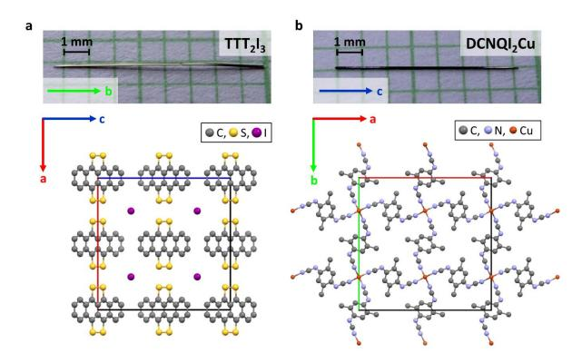
**Figure 1: Quasi-1D organic single crystals.** (a) Photograph of a macroscopic p-type  $TTT_2I_3$  single crystal together with its crystal structure showing the separated molecular stacks. (b) The same is illustrated for the investigated crystalline n-type organic conductor  $DCNQI_2Cu$ .
