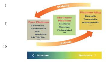
Fig. 1 Groupings of Pt-based electrocatalysts for ORR in PEM fuel cells.
