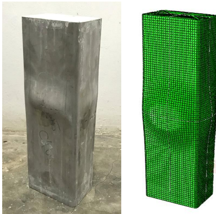
Fig. 7. Experimental and numerical failure modes for CFHSST stub specimen RHS 150×100×5-C40.
