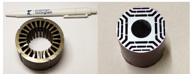
Fig. 9: Stator and rotor lamination stacks before winding and assembling (pictures are not shown in the same scale)
