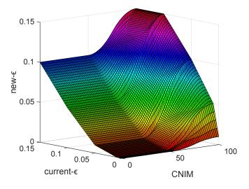
Fig. 3. Control surface of fuzzy system used to control  $\epsilon$  in XD-TA-3.
