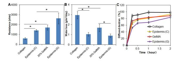
**Figure 5.** Resistance measurements (A), rate of water loss (B), and relative water permeability of naked collagen, collagen covered with a reconstructed epidermis (Epidermis (C)), GelMA hydrogel (20%), and GelMA hydrogel covered with epidermis (Epidermis (G)). Note the significant influence on barrier function of an epidermal cover. \* indicates p < 0.05.
