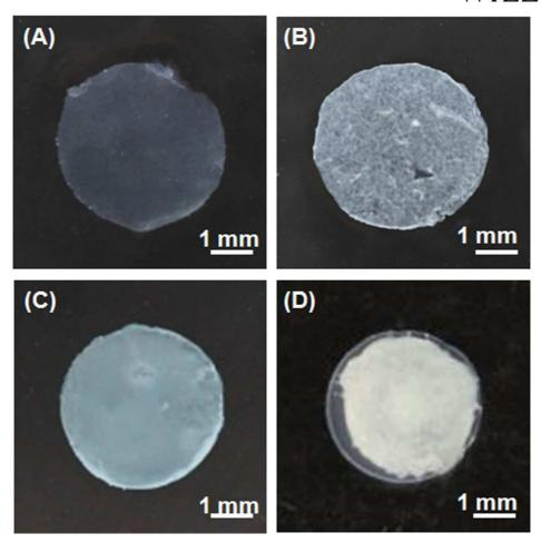
**Figure S2.** Photographs of GelMA surfaces (20%) covered with no cells (A), by a cell monolayer after submerged culture for 7 days (B), and by cell multi-layers after culture at air-liquid interface for 2 weeks (C) and 6 weeks (D).
