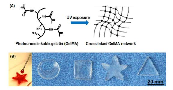
**Figure S1.** (A). Formation of crosslinked hydrogel network of GelMA. (B). Photographs showing injection of a GelMA solution (20%) via a conventional 27- gauge needle into a mould and formation of hydrogels with various shapes (round, square, star and triangle) after UV polymerization.
