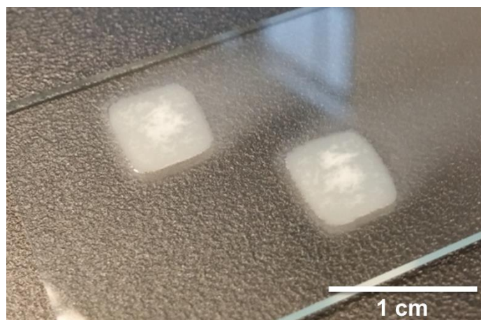
Figure 1. Images of 2 features printed from polymer 5c . Each feature represents 700 layers and was allowed to dry in ambient conditions over night before the material fully solidified.
