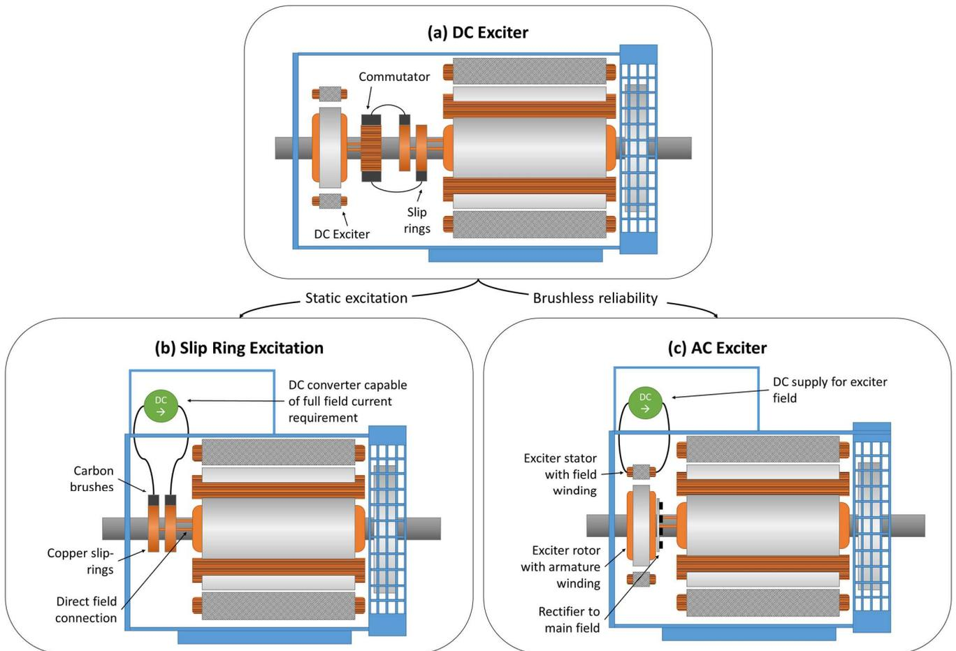
Fig. 2. Evolution of conventional excitation systems with main components of each, (a) direct coupled DC exciter, (b) static excitation through slip rings, and (c) the brushless AC exciter.
