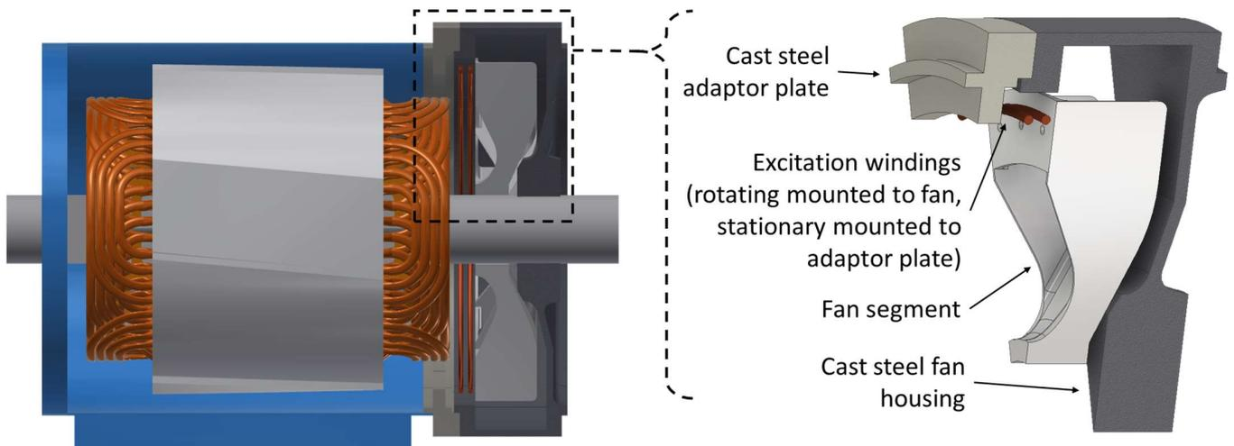
Fig. 5. Rendering of an inductive WPT ES that integrates with the existing fan and housing.
