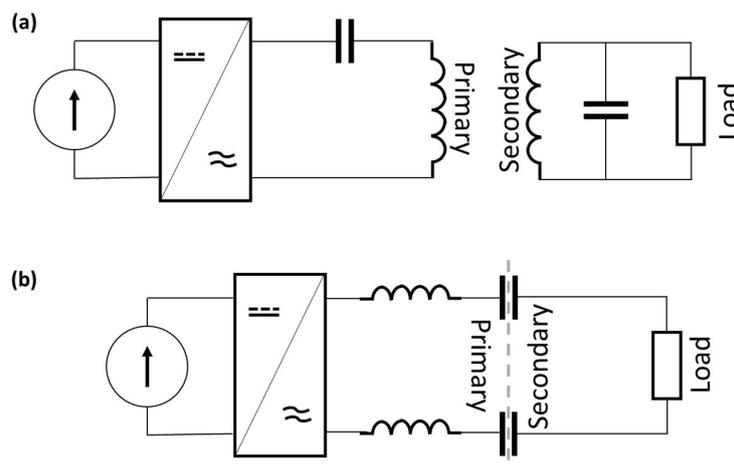
Fig. 4. WPT circuit topologies: (a) inductive with series-parallel compensation network, (b) capacitive.
