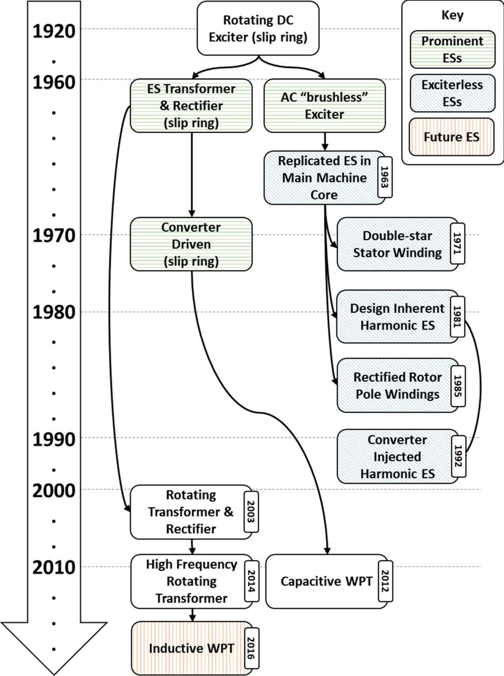
Fig. 6. Evolution of the synchronous generator ES over the past century, highlighting the prominent methods of today, the discussed exciterless methods (including the year first presented in the literature), and the future.
