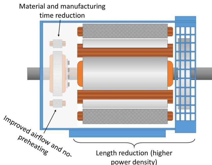
Fig. 1. Diagram of a typical synchronous generator with a rotational exciter showing the potential benefits of exciterless solutions.
