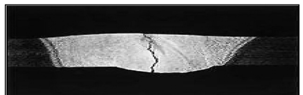
Fig. 5. Centre-line cracks in AA6082 plate/4043 filler metal TIG weld [25].
