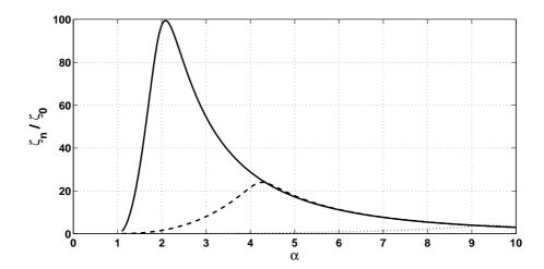
Figure 3: The impact of  $\eta$  on the damping ratio enhancement  $\zeta_n/\zeta_0$  of the suggested oscillator with  $m_2$ =0:  $\zeta_0$ =0.1 (···),  $\zeta_0$ =0.01 (--),  $\zeta_0$ =0.001 (-). All computations conducted with  $\varepsilon$ =5%.
