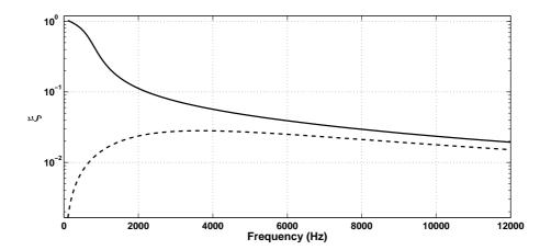
Figure 15: Damping ratio of the predicted flexural motion of the modified layered beam around z axis when  $\eta$ =0.1: With  $m_2$ =0 (–), With  $m_2$ =0.3 $m_f$  (––)
