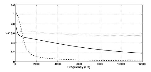
Figure 14: Damping ratio of the predicted flexural motion of the modified layered beam around z axis: With  $\eta=10$  (···), With  $\eta=1$  (-), With  $\eta=0.1$  (--)
