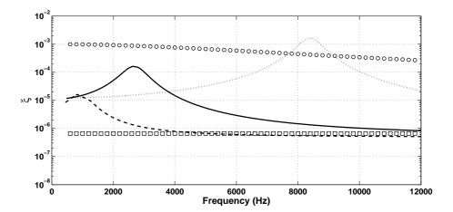
Figure 11: Damping ratio  $\xi$  as a function of frequency for the waves propagating within the beam for  $\eta$ =0.1. Result for no negative stiffness ( $\square$ ) and modified configuration with  $m_2$ =0 ( $\circ$ ). Results for:  $m_2$ =0.3M (--),  $m_2$ =0.03M (-),  $m_2$ =0.003M ( $\cdots$ ).
