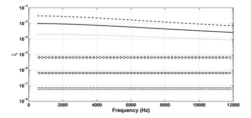
Figure 8: Damping ratio  $\xi$  as a function of frequency for the flexural wave propagating within the beam. Results for the SDoF oscillator:  $\eta$ =0.01 ( $\Box$ ),  $\eta$ =0.1 ( $\circ$ ),  $\eta$ =1 ( $\circ$ ). Results for the mechanism having negative stiffness inclusions:  $\eta$ =0.01 and  $\alpha$ =1.2 ( $\cdots$ ),  $\eta$ =0.1 and  $\alpha$ =1.6 (-),  $\eta$ =1 and  $\alpha$ =3 (--).
