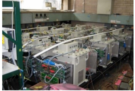
Figure 5. 3-Phase, 7-Level CHB Back-To-Back converter.
