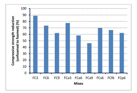
380 Fig. 11. Compressive strength reduction (%) of unfoamed to foamed concrete for the same mixes
