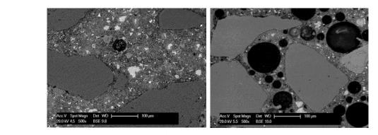
Fig. 1. SEM images for 1600 kg/m<sup>3</sup>, (left) mix without foam, (right) foamed concrete mix
