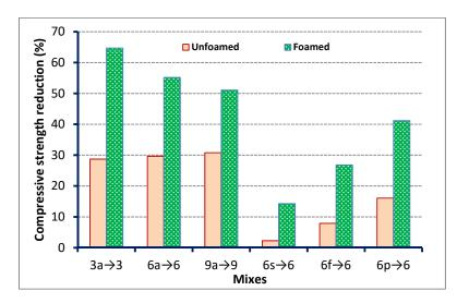
Fig. 12. Compressive strength reduction (%) of unfoamed and foamed concrete mixes (from with additives to conventional)
