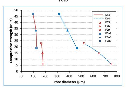
Fig. 6. Compressive strength versus void size parameters
