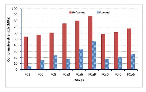
Fig. 10. 28-day Compressive strength of unfoamed and foamed concrete mixes
