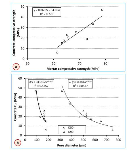
Fig. 13. (a) Mortar strength and (b) pore size parameters versus foamed concrete strength for all
