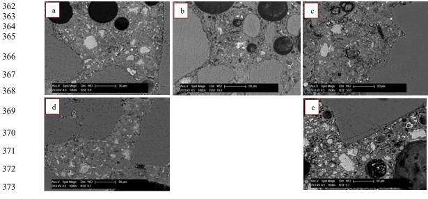
Fig. 9. Effect of additives on the cement paste microstructure a) FC6 b) FCs6 c) FCf6 d) FCp6
