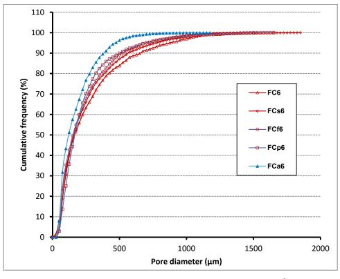
Fig. 4. Cumulative frequency (%) of pore diameters of  $1600 \text{ kg/m}^3$  mixes
