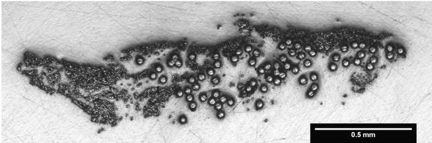
Figure 3: Optical microscope picture of the original carbon/PA6 commingled fibre tow.
