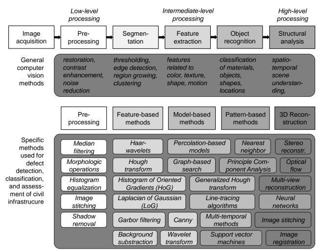
Figure 1: Categorizing general computer vision methods (top) and specific methods to defect detection, classification and assessment of civil infrastructure.
