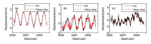
Fig. 8. The fitting results of external load of air temperature (a), water level (b) and other factors(c) after modelling the ICs.
