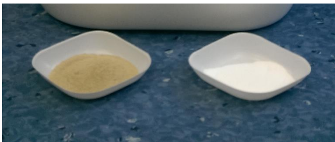
Figure 7 Photograph of a commercial sample of MIL-53(Al) (left), and our scaled-up material prepared by continuous flow (right).
