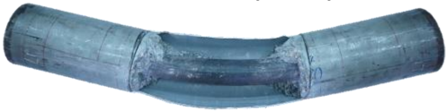
(b) Concrete cracking and crushing
