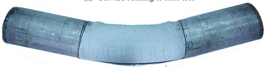
(a) Outward buckling of outer tube
