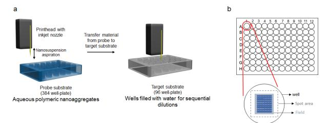
**Figure S2.** (a) Printing process by focusing on the nozzle setup. On the left-hand side, the aqueous polymeric nanosuspension/aggregation aspiration. On the right-hand side, printing dispensing of the aspired nanoaggregates into wells filled with 200  $\mu$ L of water. (b) the 96-well plate target substrate, detailed view of a well with designed spot area and field, selected print pattern with adjustable number of drops per spot in magnified view.
