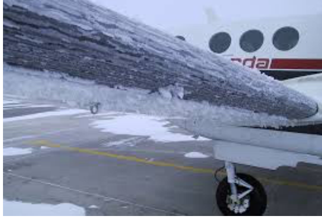
Figure 1: Ice accumulation on the wing of an aircraft. Adapted and reprinted with permission from reference [22].
