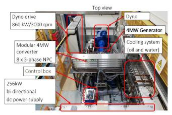
Fig. 15: High power area test facility: 860kW dynamometer and test rig layout.
