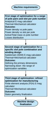
Fig. 4: Machine optimisation flowchart.
