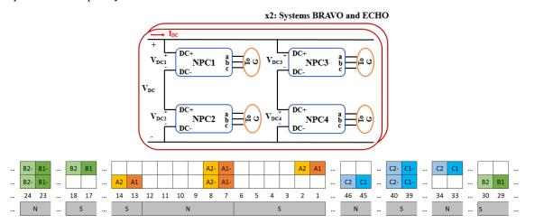
Fig. 9: Full 8x3-phase converter comprised of two 3 kV DC-Link channels and 8x3-phase winding layout
