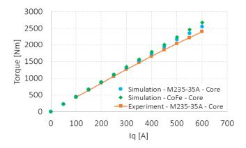
Fig.18: Torque-current characteristic at 500rpm, 800Vdc.
