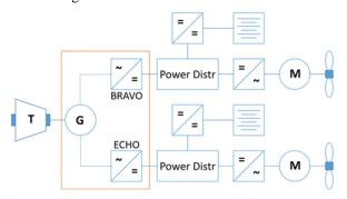
Fig. 1 Schematic of the drive train system. Component 'G' is the electrical machine (Generator) and BRAVO and ECHO are two channels of the converter, which is connected to the power distribution system.
