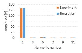
Fig.16: Line-to-line bEMF harmonic spectrum at 2000 rpm.
