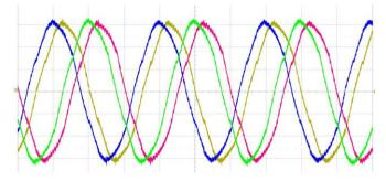
Fig.19: The acquired phase current waveforms at the motoring mode (Iq = 600Apk, 500rpm, 2400Nm, 800Vdc); Ch1 yellow: echo-npc2-phB, Ch2 red: echo-npc2-phC, Ch3 blue:bravo-npc2-phB, Ch4 green: bravo-npc2-phC; ); x and y axes are time [ms] – 10ms/div and current [A] – 200 A/div, respectively.
