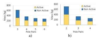
Fig. 8: Mass segregation variation with pole pair; (a) -1 SPP; (b) -2 SPP.
