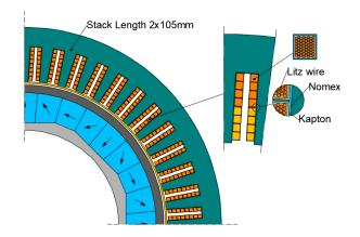
Fig. 13: Schematic of the final machine design.
