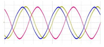
Fig.17: Measured line-to line bEMF waveforms at 2000rpm (Ch1 - yellow - bEMF<sub>AB</sub>-echo, Ch2 - red - bEMF<sub>BC</sub>-echo, Ch3 - blue – bEMF<sub>AB</sub>-bravo); x and y axes are time [ms] (50 ms/div) and voltage [V] (50 V/div), respectively.
