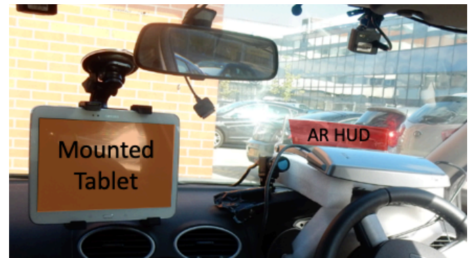
Fig. 2. Experiment setup. The AR HUD (right) was fixed to the dashboard and adjusted to the user's line of sight. A color palette was also displayed using a tablet mounted at eye level (left) of the driver, simulating a large tablet-style in-vehicle display.
