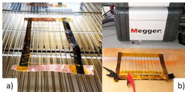
Fig. 4. Twisted pair specimens, a) thermal aging in environmental chamber, b) AC electric withstand test.
