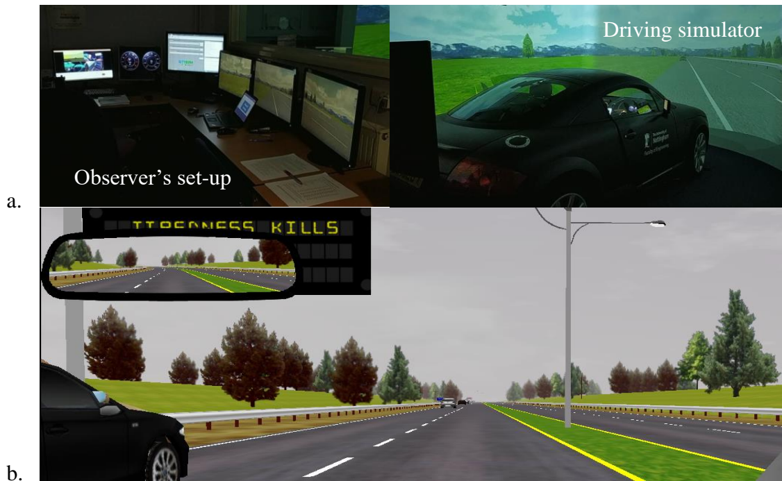
1 2 Figure 1 Experimental set-up: a. Driving Simulator and b. design view of dual carriageway 3 All participants drove in both the driving conditions (with and without VA) in a 4 counterbalanced order to avoid any learning effects. A general layout of the experiment design 5 and protocol is illustrated in Figure 2.
