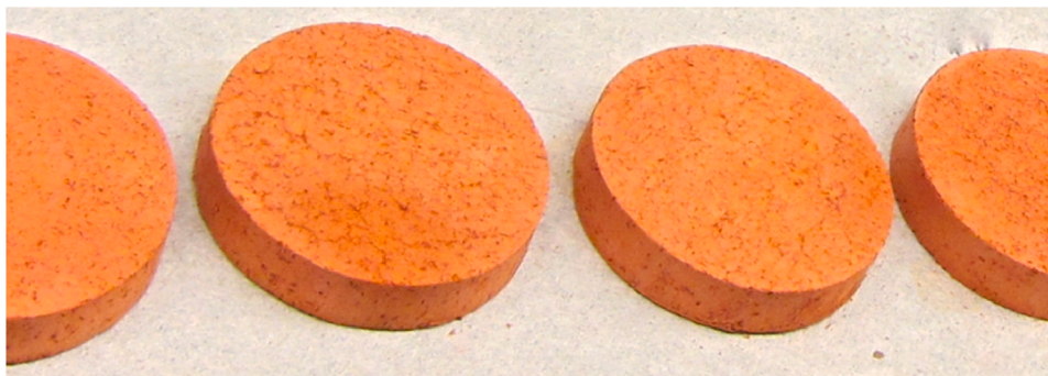
Fig. 57. Schematic of disc-shape porous ceramic filter containing Ag nanoparticles for point-of-use water treatment. Reproduced with permission [276]. Copyright 2013, American Chemical Society.
