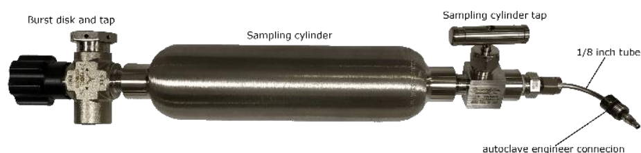
Fig. 2. Cylinder system used to obtain on-line samples during monitoring experiments. Swagelok product codes: burst disk and tap: SS-16DKM4F4-A-2, sampling cylinder: 36L-50DF4-150-T, sampling cylinder tap: SS-20VM4-F4
