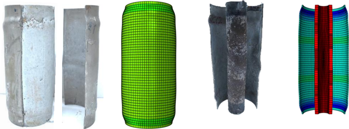
(c) Outward local buckling of outer tube
