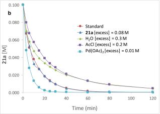
**Figure 1.** Probing the effect of acid chloride hydrolysis on global kinetics by carrying out different ["excess"] experiments in conjunction with a "pre-mix" addition experiment.
