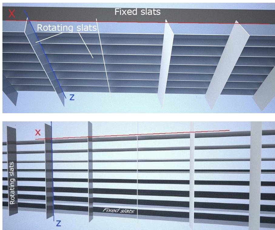
Figure 9: Two-layer parametric louver system
