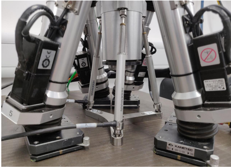
Fig. 6. Frame and double ball-bars for the calibration of Free-Hex.
