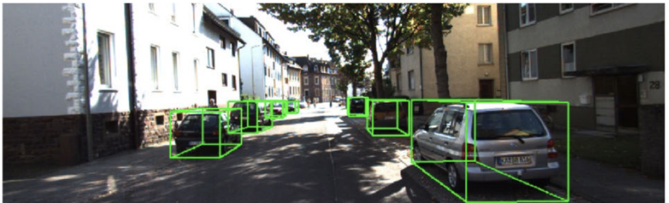
FIGURE 11. Example 3D detection result from the KITTI validation set projected onto an image. Image from Sindagi et al. [297].
