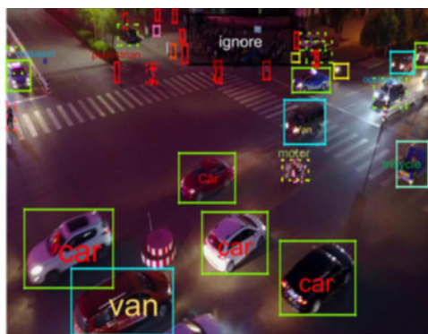
FIGURE 6. A drone-based image with bounding box and category labels of objects. Image from VisDrone 2018 dataset [7].
