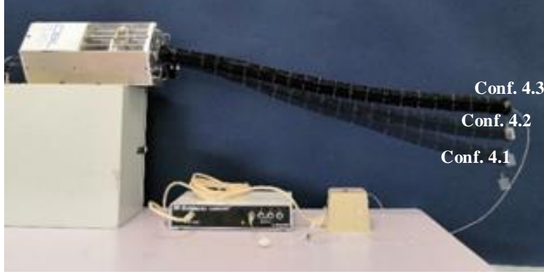
Fig.14 Physical demonstration of the stiffness adjustment under 100g end load
