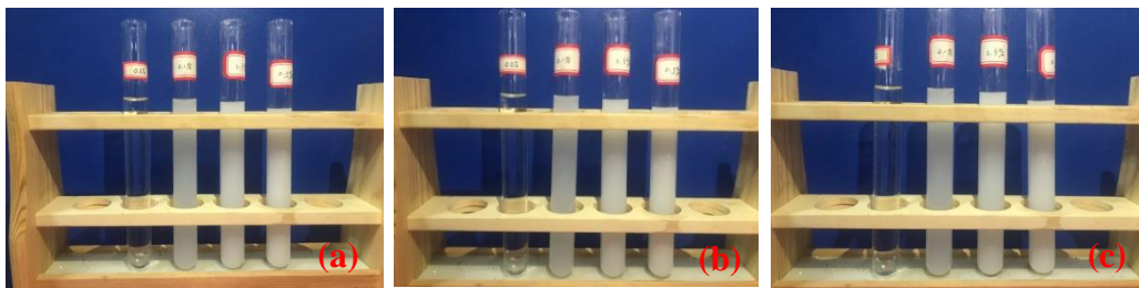
Fig. 2. \text{SiO}_2 -water nanofluids at different quiescent time, (a) just prepared, (b) laying up 10 days, (c) laying up 20 days
