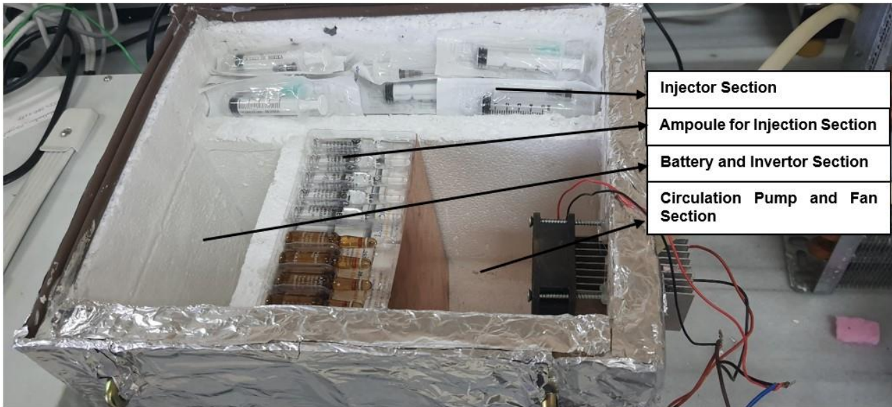
Figure 2 Schematic description of vaccine cabinet
