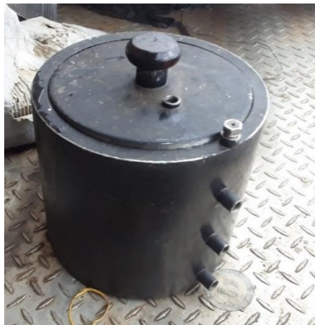
Figure 2 A photograph of the finned storage cooking pot
