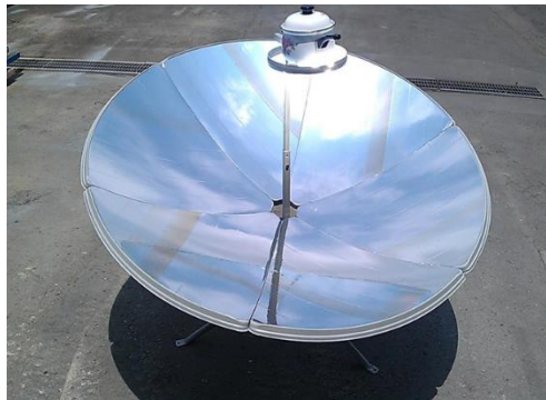
Figure 3 A photograph of the 1.8 m parabolic dish solar cooker with a silvered cooking pot containing water as the test load
