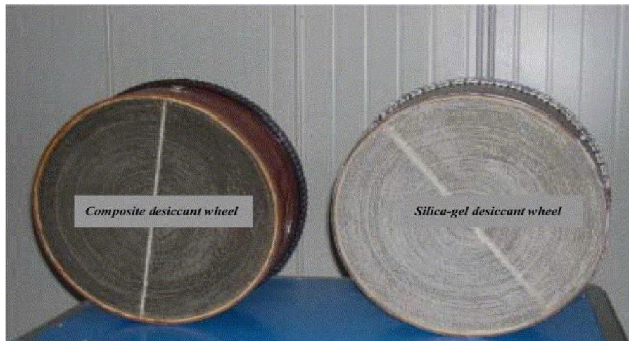
Figure 5 Pictures of the developed composite and SG-based RDW (Jia et al., 2007).
