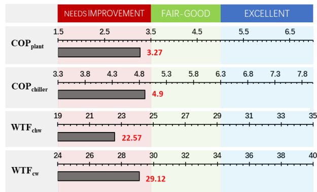
Figure 7 Average summer chiller plant efficiency in kW/kW (COP). Input energy includes chillers, pumps, and tower fans.
