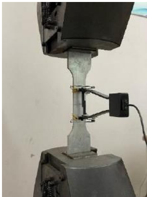
Fig. 1. Test set-up for longitudinal tensile coupons
