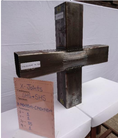
(c) Test vs FE comparison for chord side wall failure (S) mode of 90° RHS X-joints.
