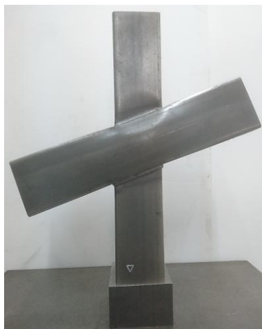
(b) Test vs FE comparison for combined failure (F+S) mode of non-90° RHS X-joints.
