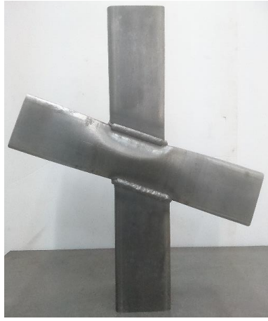
(c) Test vs FE comparison for chord side wall failure (S) mode of non-90° RHS X-joints.
