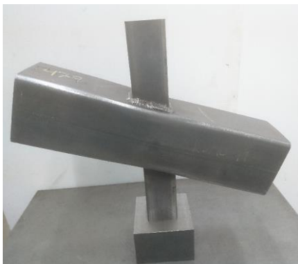
(a) Test vs FE comparison for chord face failure (F) mode of non-90° RHS X-joints.
