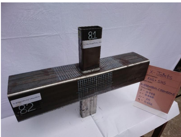
(a) Test vs FE comparison for chord face failure (F) mode of 90° RHS X-joints.
