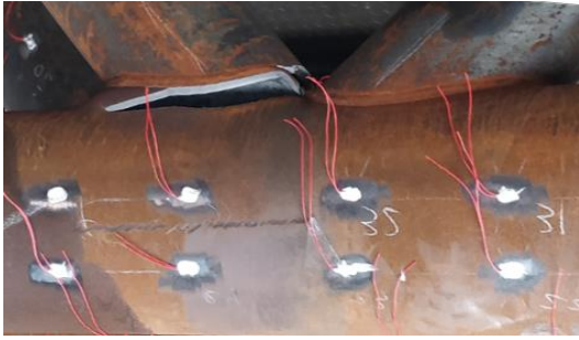
(a) Punching shear failure of chord
