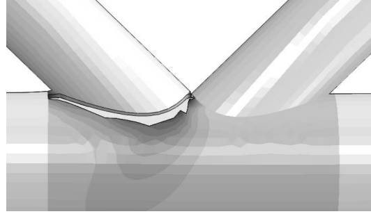
(a) Punching shear failure of chord
