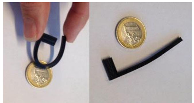
Fig. 27. 3D printed flexible antenna enabled by LM [178].
