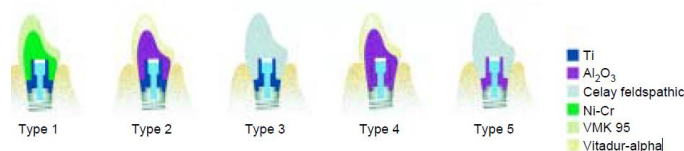
Fig. 57 Design of tested implant restorations (1) metal-ceramic crowns cemented to titanium abutments, (2) In-Ceram crowns cemented to titanium abutments, (3) Celay feldspathic crowns cemented to titanium abutments, (4) In-Ceram crowns cemented to milled ceramic abutments and (5) Celay feldspathic crowns cemented to milled ceramic abutments [38]
