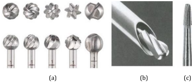
Fig. 42. Bone milling tools of different shapes: (a) round fluted, (b) pear, (c) cross cut fissure [171].
