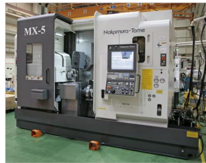
Fig. 65. Multi-tasking machine tools based on turning center (Source: Nakamura-Tome Precision Industry Co., Ltd.)
