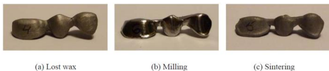
Fig. 54 (a) Co-Cr fixed partial denture made using the lost wax technique, (b) milling and (c) selective laser sintering [70].
